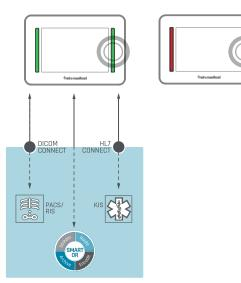
When a patient is brought into the induction room, all necessary and previously defined data is transferred directly from the HIS to the client. Here the procedure is created and transmitted back to the KIS via HL7 message. When the patient leaves the operating room after the procedure, DOORSIGN changes the background colour and shows what happens next.
